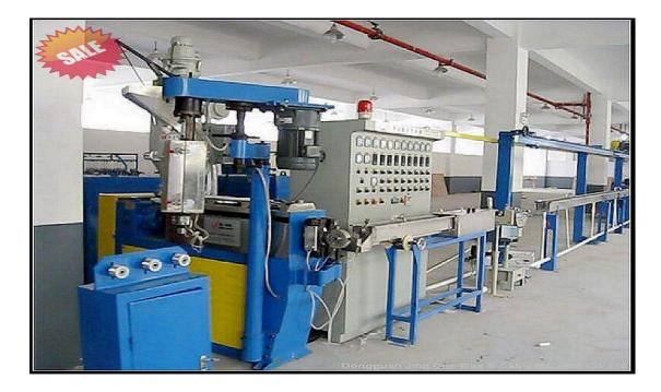
$\rm I$  .Application: Suitable for PVC, LDPE, XLPE, LSHF, TPU etc. Insulation material of the wire and cable monochrome, double-color, double-layer, tri-layer extrusion working.
