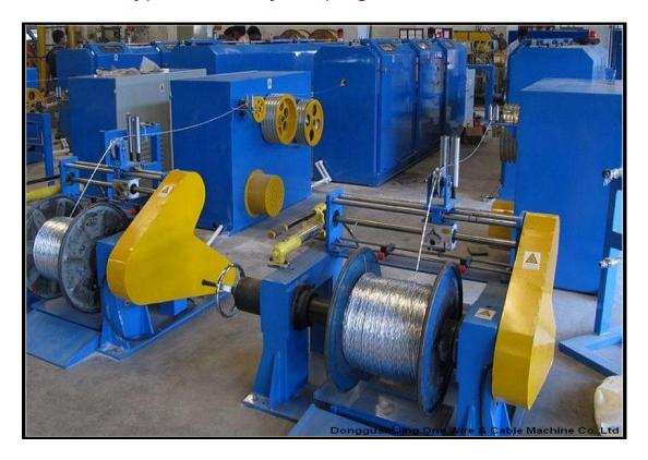
The machine is horizontal double-layer wrapping machine(paper tape, aluminum foil)with rotation plate wrapping on the core wire, own single wrapping head. Mainly uses for the electric wire, the strength cable, controls cable and optical cable etc. insulated wire core mica tape wrapping, the fireproof electric wire electric cable mainly is suitable for power plant, airport, ships, high rise construction, subway, underground street and recreation area.
