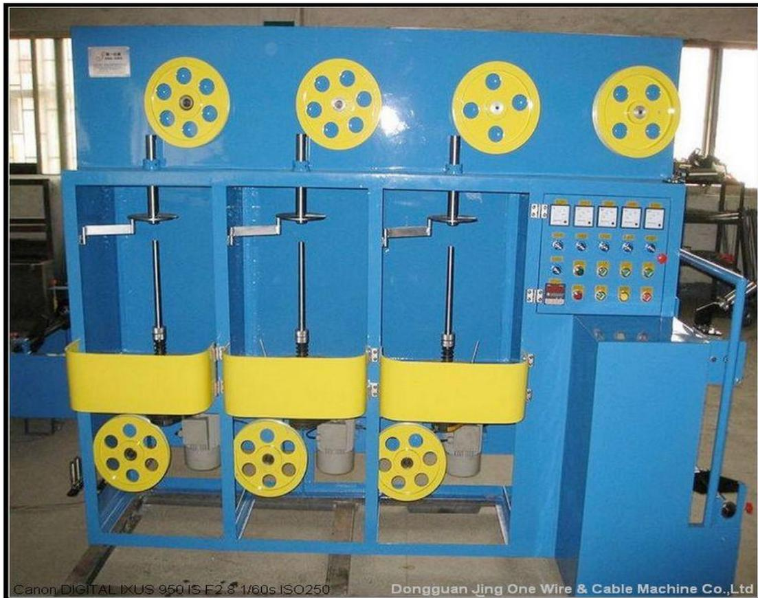
The machine is vertical three-layer wrapping machine(paper tape, aluminum foil)with rotation plate wrapping on the core wire , own single wrapping head . Mainly uses for the electric wire, the strength cable, controls cable and optical cable etc. insulated wire core mica tape wrapping, the fireproof electric wire electric cable mainly is suitable for power plant, airport, ships, high rise construction, subway, underground street and recreation area. It's sold well at Pakistan , UZ , Dubai .
