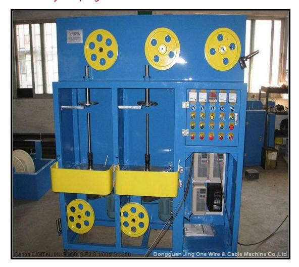
The machine is vertical double-layer wrapping machine(paper tape, aluminum foil) with rotation plate wrapping on the core wire, own single wrapping head. Mainly uses for the electric wire, the strength cable, controls cable and optical cable etc. insulated wire core mica tape wrapping, the fireproof electric wire electric cable mainly is suitable for power plant, airport, ships, high rise construction, subway, underground street and recreation area. It's sold well at India, Pakistan, UZ, Dubai.
