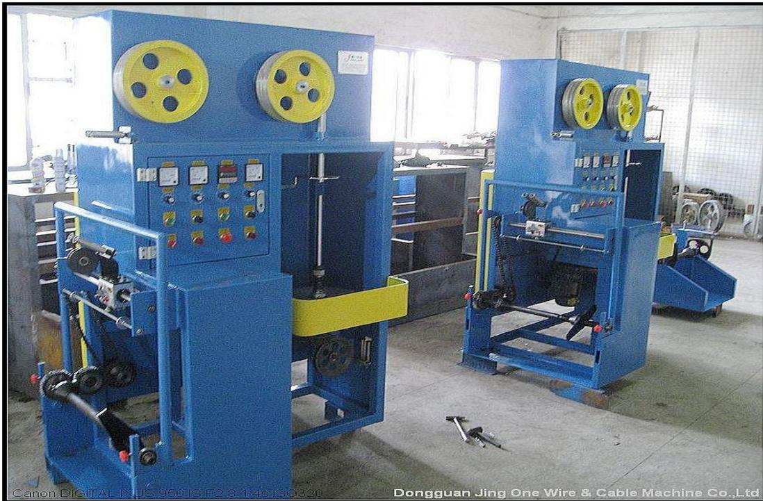
The machine is vertical single-layer wrapping machine(paper tape, aluminum foil)with rotation plate wrapping on the core wire, own single wrapping head. Mainly uses for the electric wire, the strength cable, controls cable and optical cable etc. insulated wire core mica tape wrapping, the fireproof electric wire electric cable mainly is suitable for power plant, airport, ships, high rise construction, subway, underground street and recreation area. It's sold well at India, Pakistan, UZ, Dubai.
