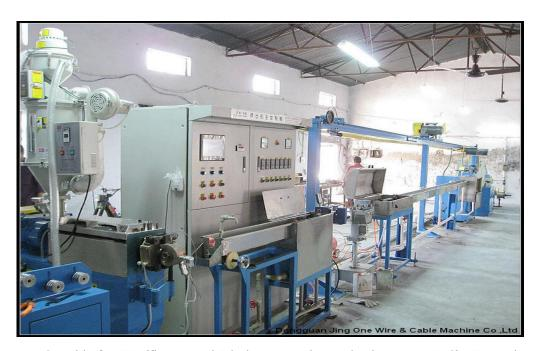
Application: Suitable for FEP (fluorinated Ethylene Propylene, also known as F46), FPA and ETFE (also known as F40) etc. fluorine plastic production.
