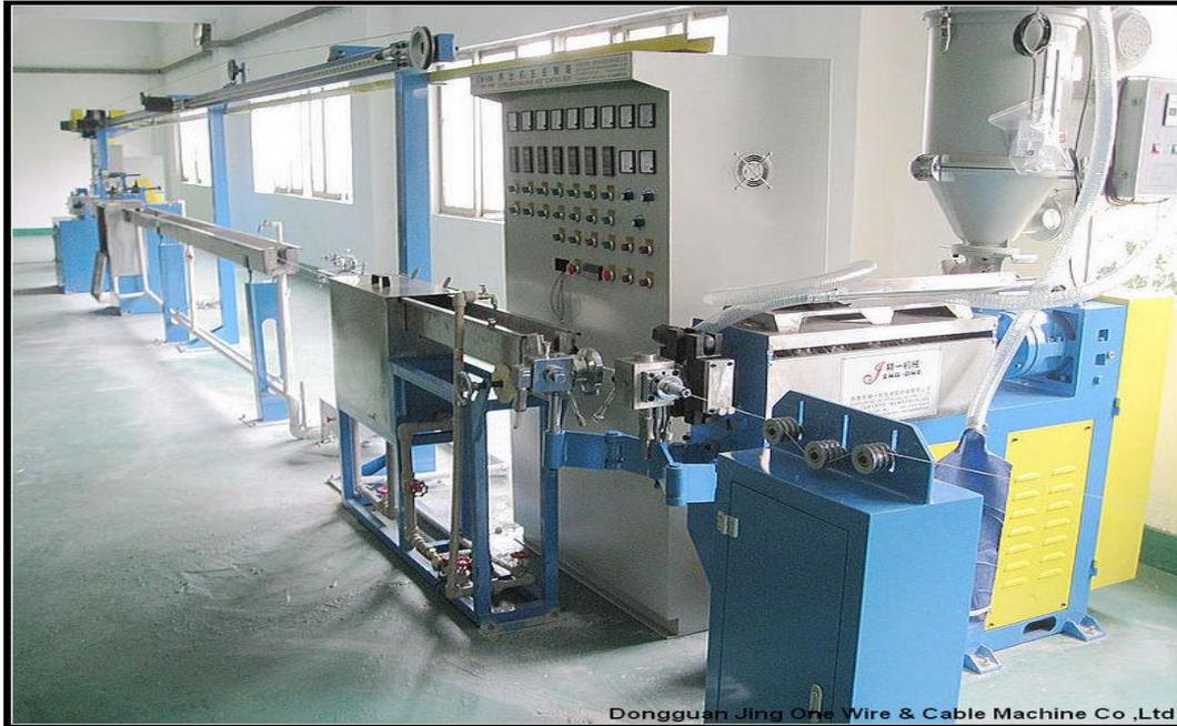
Application: Suitable for PVC, PU and PE etc. plastic extrusion, mainly used for UL electric wire production.
