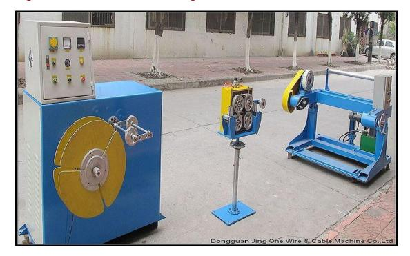
Big High speed automatic traverse coiling machine is used for 50-240mm<sup>2</sup> single wire and wire diameter less than 30mm round jacketing coiling and traverse. The product includes pay-off, measurement accuracy and big cross section high speed automatic coiling machine.
